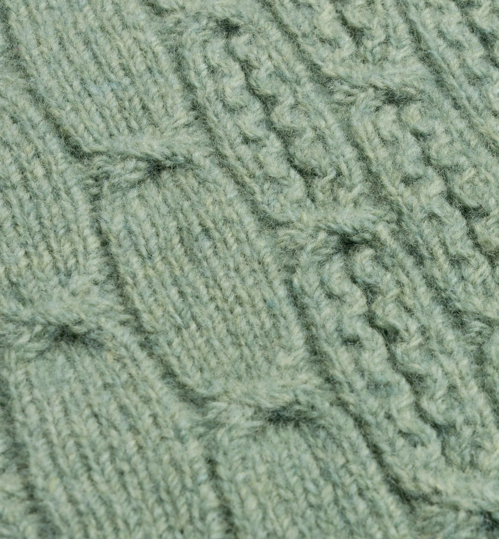
2210026 | Women's Fully Fashion Turtleneck Pullover that examines the perception of color in different sized cross-cable structures. The garment was designed fully digitally with k.innovation CREATE DESIGN and external 3D software before the final knitting program with k.innovation CREATE PLUS was executed. | ADF 530-24 ki multi gauge | E 3,5.2
