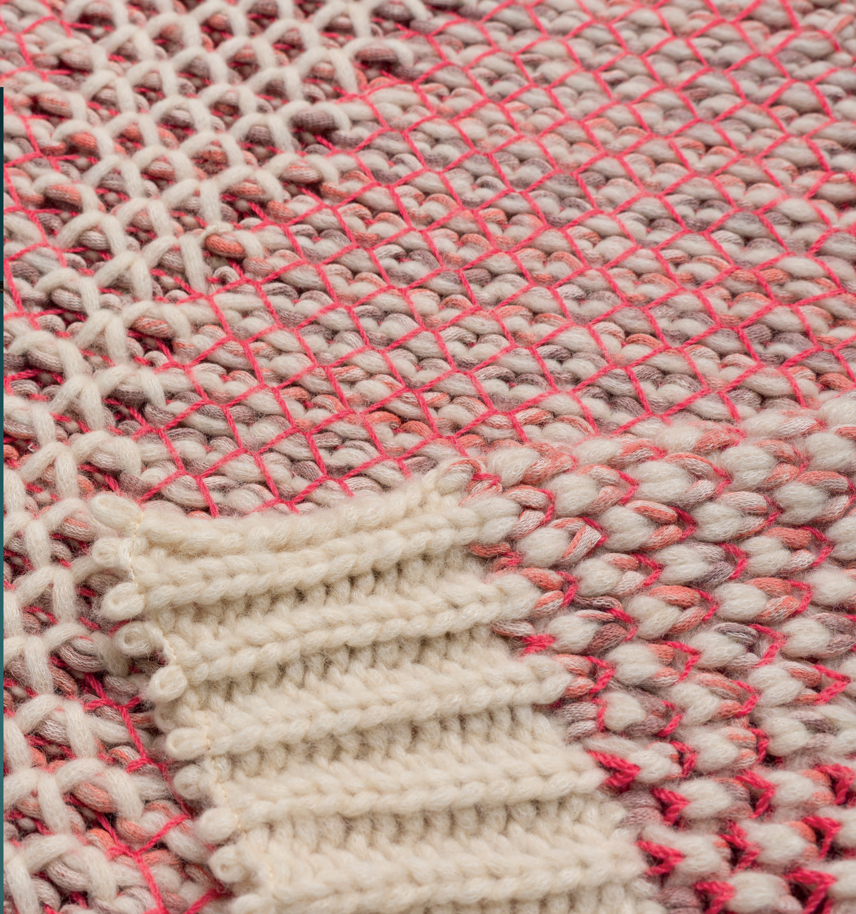
2310002 | Women's Coarse Gauge Poncho with sophisticated tuck structure using three different yarn gauges to create multifaceted compositions of color and structure. This poncho is knitted jointlessly in 1x1 technique starting with the rib collar. | CMS 520 C+ ki multi gauge | E 1,5.2
