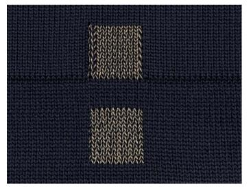
Textile switch: selective plated sections can be overlapped to close the circuit
