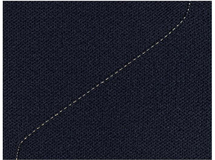
**Inserting of conductive wire**
