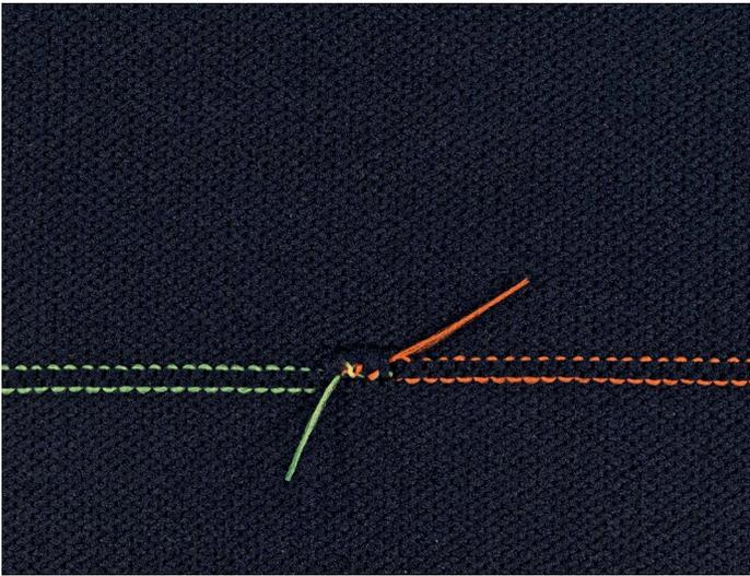
**Connecting two or more conductive wires by Selective Plating**
