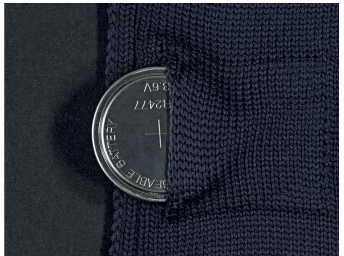
**Textile socket in tubular and Selective Plating technique**
