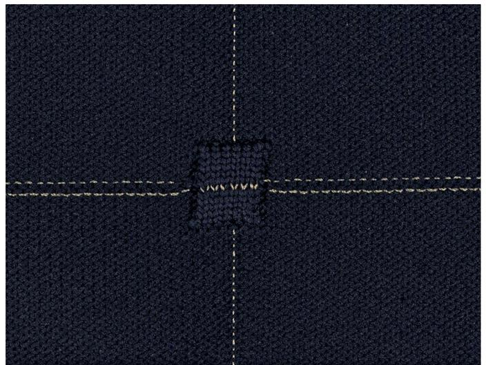
**Shield-off single crossing conductive wires**
