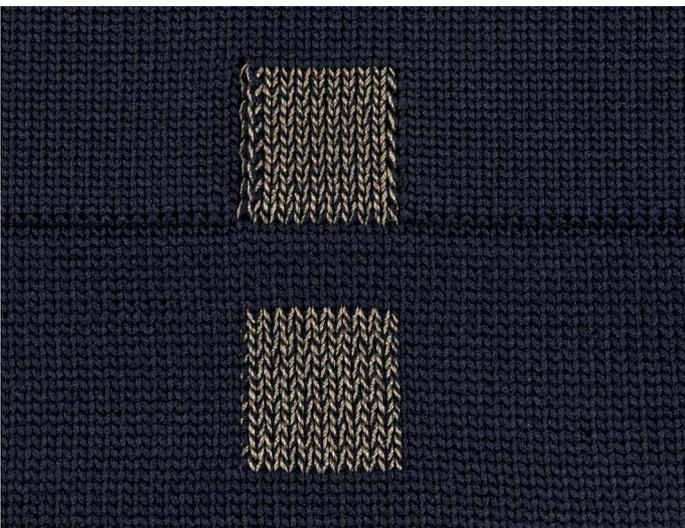
**Textile switch: selective plated sections can be overlapped to close the circuit**
