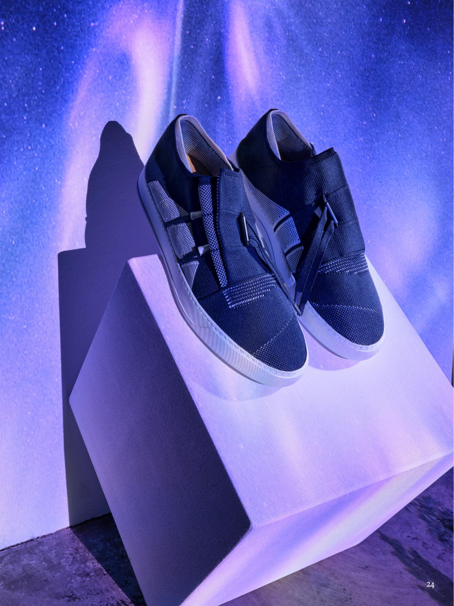
Knitted shoe upper with pleat closure design on the dorsum of the foot which is integrated directly in the machine with maximum racking effect and has knitted-on straps to enhance stability. The sustainable version of the shoe upper is knitted with Deja™ – 100% recycled polyester yarn by Indorama Ventures and eco-friendly dyed with DyeCoo's innovative CO<sub>2</sub> technology without the use of water and process chemicals.
