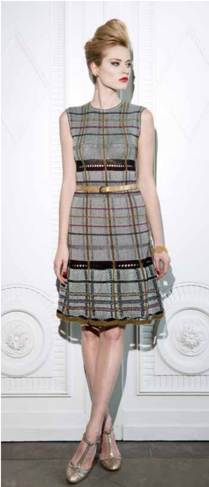
1110046 · CMS 822 HP MULTI GAUGE · E 7.2 Stoll-multi gauges® Tartan intarsia dress with 18 (20) intarsia yarn carriers and transfer structure on jersey, knitted in one piece with three different gauge optics Knitting Time: 1 piece: 32:00 min – 0,8 m/s
