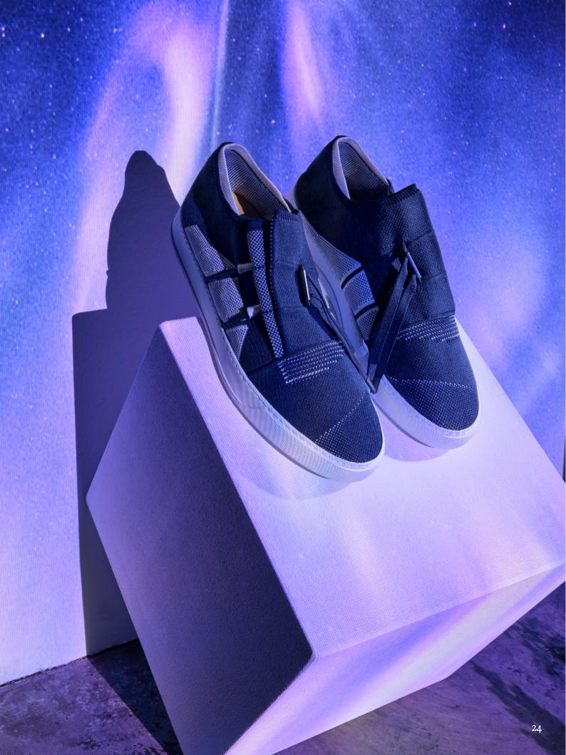
Knitted shoe upper with pleat closure design on the dorsum of the foot which is integrated directly in the machine with maximum racking effect and has knitted-on straps to enhance stability. The sustainable version of the shoe upper is knitted with Deja<sup>™</sup> – 100% recycled polyester yarn by Indorama Ventures and eco-friendly dyed with DyeCoo's innovative CO<sup>2</sup> technology without the use of water and process chemicals.
